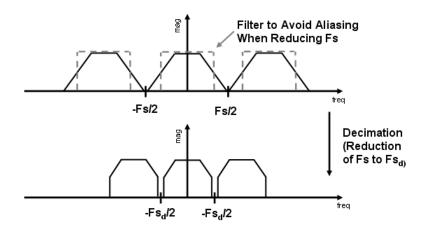
An analogous approach must be taken to avoid *imaging* when performing interpolation on a sampled signal. For more information about the effects of decimation and interpolation on a sampled signal, refer to any one of the references in the "Bibliography" section of the Filter Design Toolbox User Guide.
